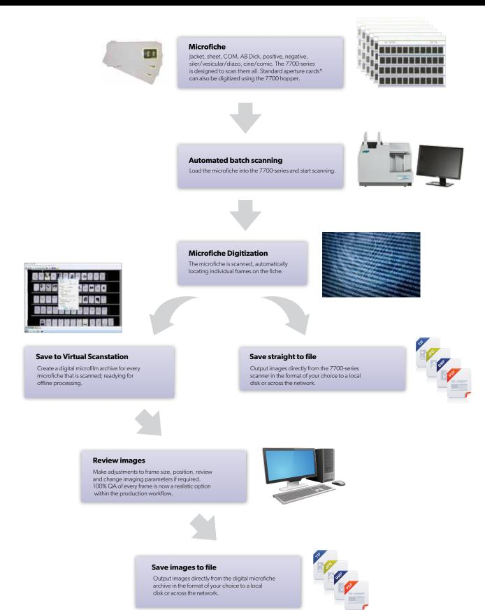
\*The 7700 scans images from the aperture window, but does not read Hollerith code. If Hollerith reading is required, consider the Wicks and Wilson C400 aperture card scanner.
