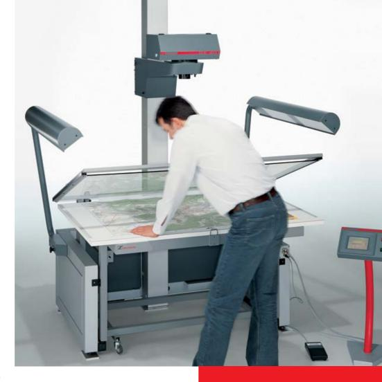
**Options:** Kit for color filming, front edge positioning of original acheived by automatic positioning of camera tables (only for A1/D-size tables), automatic fade-in of 3-level blip, automatic fade-in of 8 alphanumeric characters (in the camera head), mobile photocell for local point-measurement, foot pedal for exposure, ergonomical footrest with integrated foot pedals for book cradle and exposure. More accessories on request
