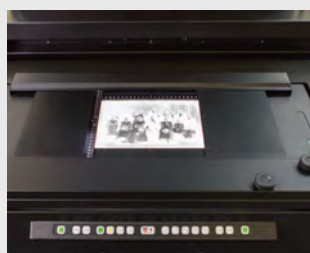
Holder for glass plates, continuously adjustable
