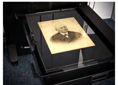
Photo table with glass plate and soft pad for very careful handling
