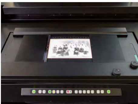
Holder for glass plates, continuously adjustable
